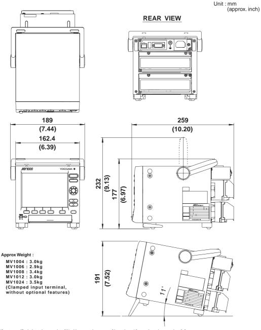
If not specified, the tolerance is  $\pm$ 3%. However, in cases of less than 10mm, the tolerance is  $\pm$ 0.3mm.
