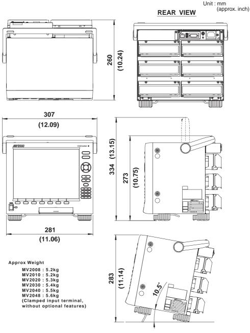
If not specified, the tolerance is ±3%. However, in cases of less than 10mm, the tolerance is ±0.3mm.
